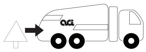
REAR END LOADER (REL): Used to collect a variety of items. (ACI uses them to collect holiday trees.) Has a hydraulic blade that compacts materials that are "loaded" by hand into the "rear end" hopper of the truck.
