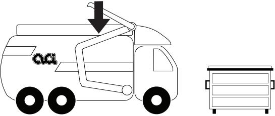
FRONT END LOADER (FEL): Used to empty bins. Has hydraulic forks that slide into the pockets of bins and lifts the bin over the "front end" of the truck to "load" (empty) bins into a hopper in the top of the truck.
