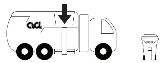
AUTOMATED SIDE LOADER (ASL): Used to empty carts. Has a hydraulic arm that "automates" the collection process and "loads" (empties) carts into a "side" hopper.
